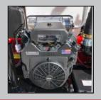
THE FT 150 VX IS POWERED BY A 25-HP KOHLER GAS ENGINE, WHICH PROVIDES AMPLE AMOUNT OF POWER TO RUN THE BLOWER AND WATER PUMP.
